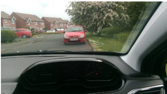
Parking on RIGHT , kerb points to PAUSE ["II"] symbol (and right handles touch kerb) Centre of road also points here when waiting, at "left of centre", to turn right
